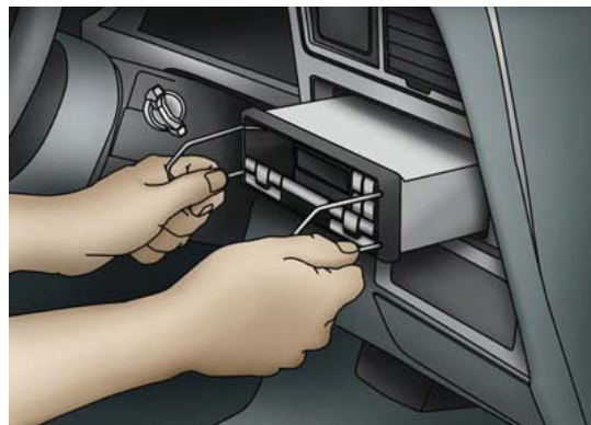
DIN tools are used to remove the factory stereo from a 2000 Ford Expedition.
