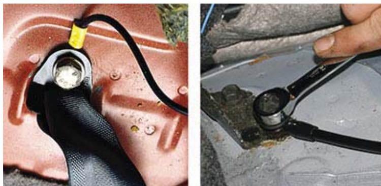
Bolt the ground terminal tightly to the vehicle's metal chassis.
