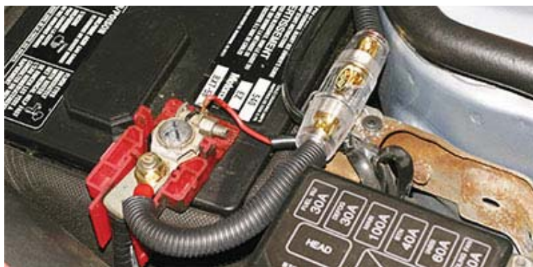
Fuse installed on power wire, and secured in engine compartment.
