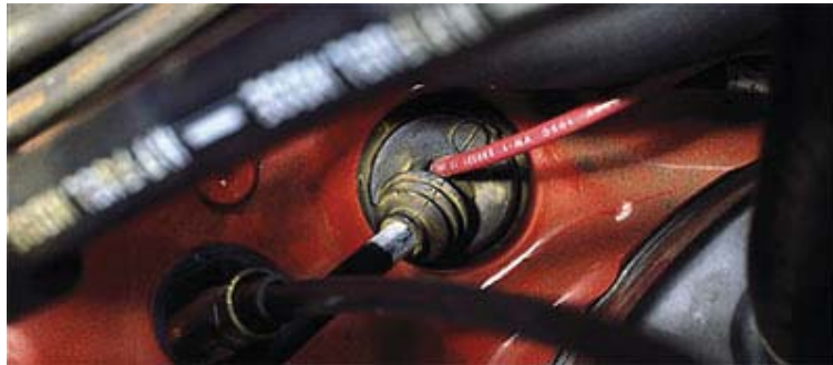
Route the red wire from your amp wiring kit through a hole in your vehicle's firewall.
