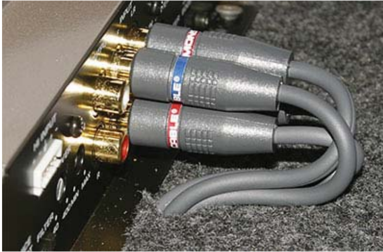
RCA cables routed through slits in the vehicle's carpet, and connected to the amplifier's signal inputs.
